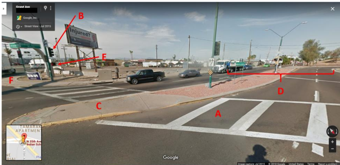
Figure 1: Image from Google Street View demonstrating the six safety features evaluated. A: High-visibility crosswalk. B: Traffic signal. C: Refuge Island. D: Number of lanes. E: Countdown pedestrian signal. F: Sidewalk.
